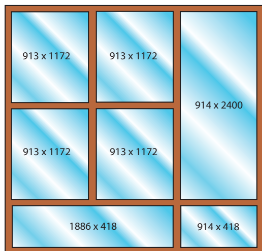
Example of assembly (in mm) Unlimited partition
